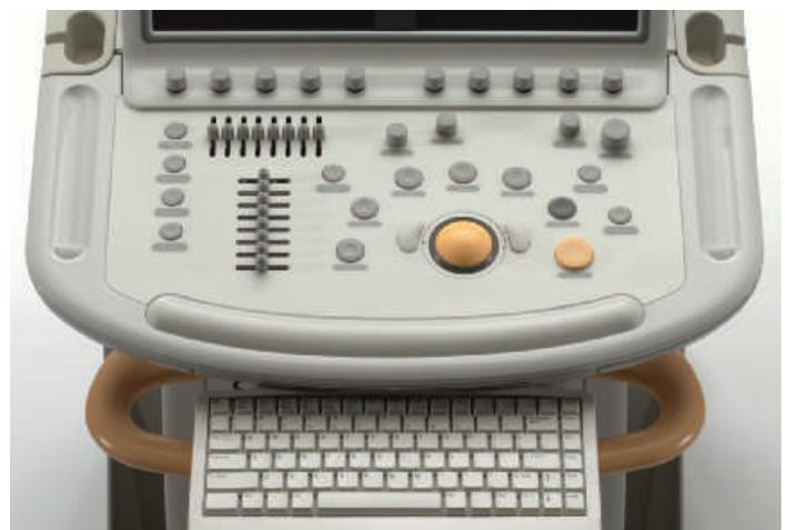
The ergo-centric iE33 control panel places primary keys for easy accessibility. It features tri-state lighting to help you while scanning in dark environments.
